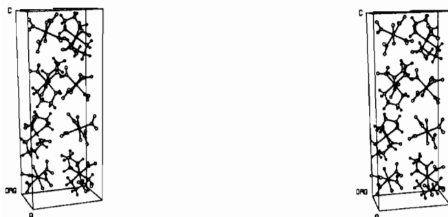
Fig. 3. Packing of the ions in the lattice. A full unit cell is shown. Note that the -\text{NO}_2 ligands of both ions are suitably oriented to form hydrogen bonds with those on either -\text{NH}_2 or -\text{NH}_3 neighbors.
